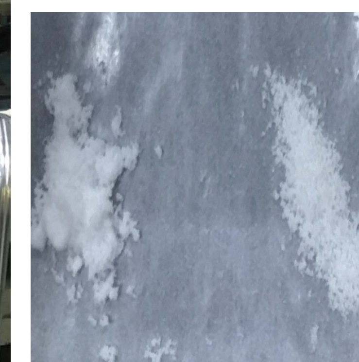
Fig.4 - LiCl before drying (L) and after drying (R). Not the decrease in volume and clumping.
