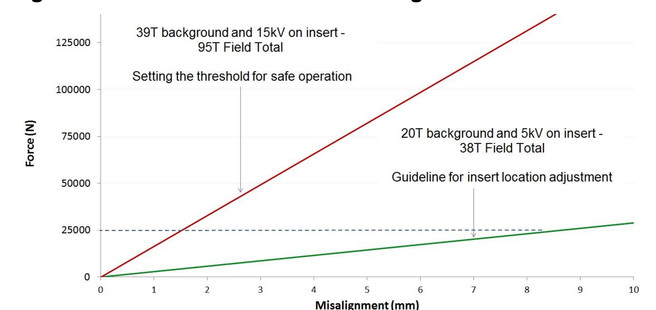
Figure 6: Force as a function of misalignment at various field
