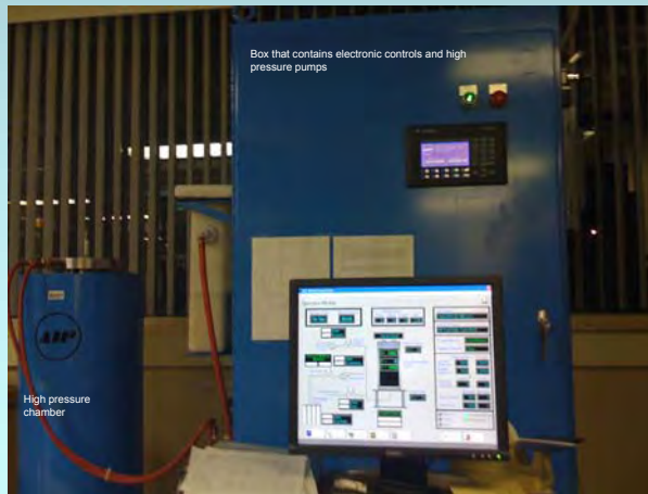
View of the hot isostatic press (HIP) unit. The maximum capabilities are ~2500 °C and 200 MPa (= ~2000 Atm = ~30,000 psi). Ar gas is used to achieve the high pressure. The high temperature is achieved using a C or Mo heating element. This HIP is a cold-wall system, which means the pressure vessel is heated on the inside and the walls are "cold". A hot-wall system has the heater on the outside of the pressure vessel and the walls are hot.
