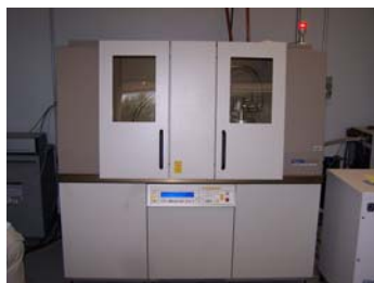
HUBER imaging plate Guinier camera 670, which was used for the x-ray diffraction experiments
