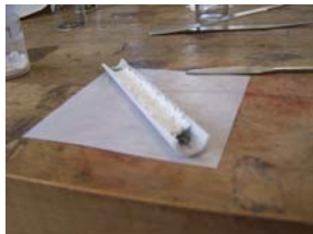
Top Left: \text{Sr}_4\text{V}_2\text{O}_{10} before it is put into the tube furnace. Top Right: \text{Sr}_2\text{VO}_4 just after burning. Bottom: \text{Sr}_2\text{VO}_4 in mortar with pestle.
