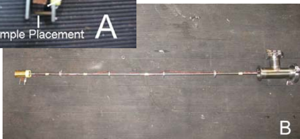
Figure 1B: This figure showcases the probe that was designed and used for this project. It features two connectors, a thermometer, and an extensometer.
