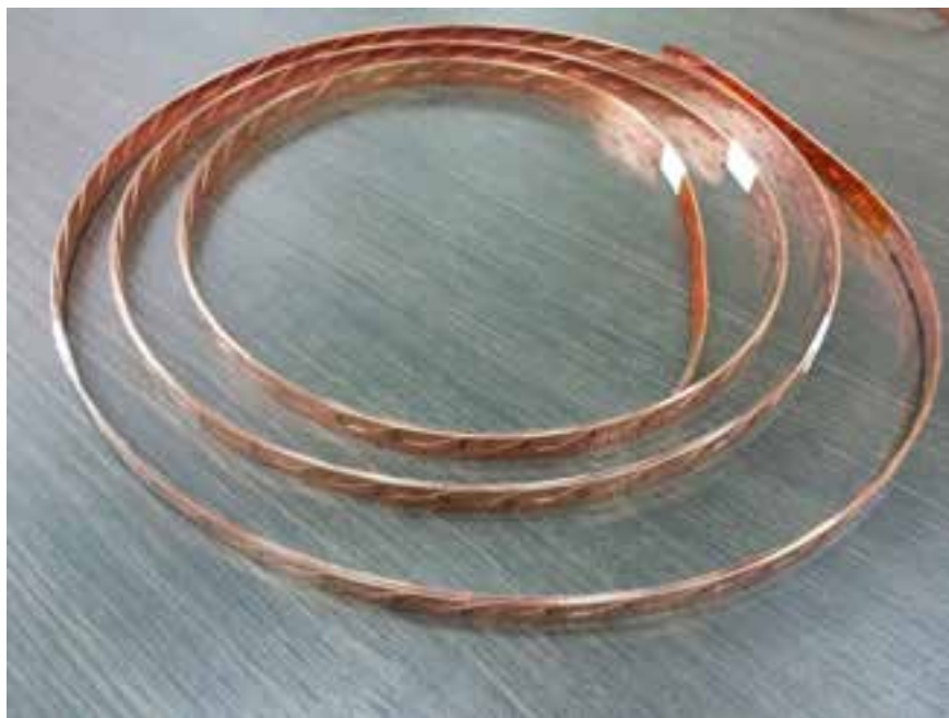
Jul 2015: 2.5 m PnC cable provided to CERN for testing
