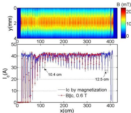
Fig.2 YateStar results of the damaged MC tape after the background magnet quenched.
