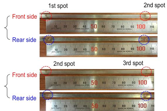
Fig.3 Pictures of the damaged spots and peel-off of stainless steel layers.
