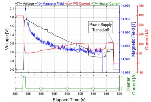
Fig.1 Quench of an LTS background magnet.
