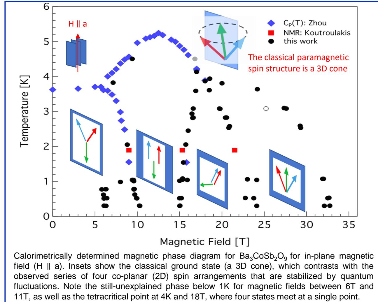
**Facilities and instrumentation used:** DC field Facility. Heat capacity measurements shown in black done in 35 T resistive magnet and dilution refrigerator. Blue points done using SCM1.
