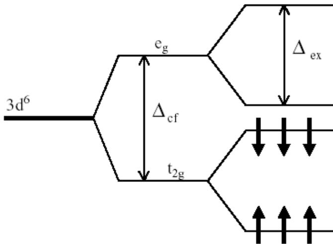
Scheme representation of various  $Co\ d^6+d^7L$  configurations in different spin states:
