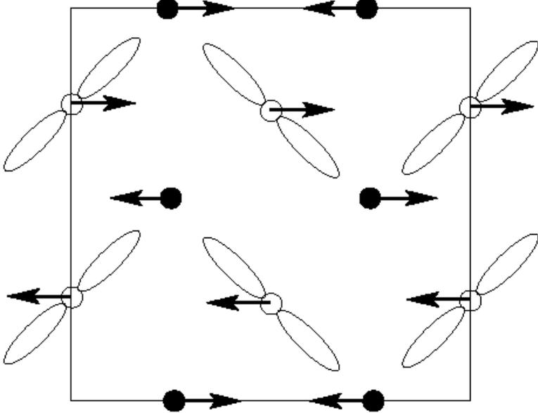
Orbital order for partially filled  $e_g$  shell
