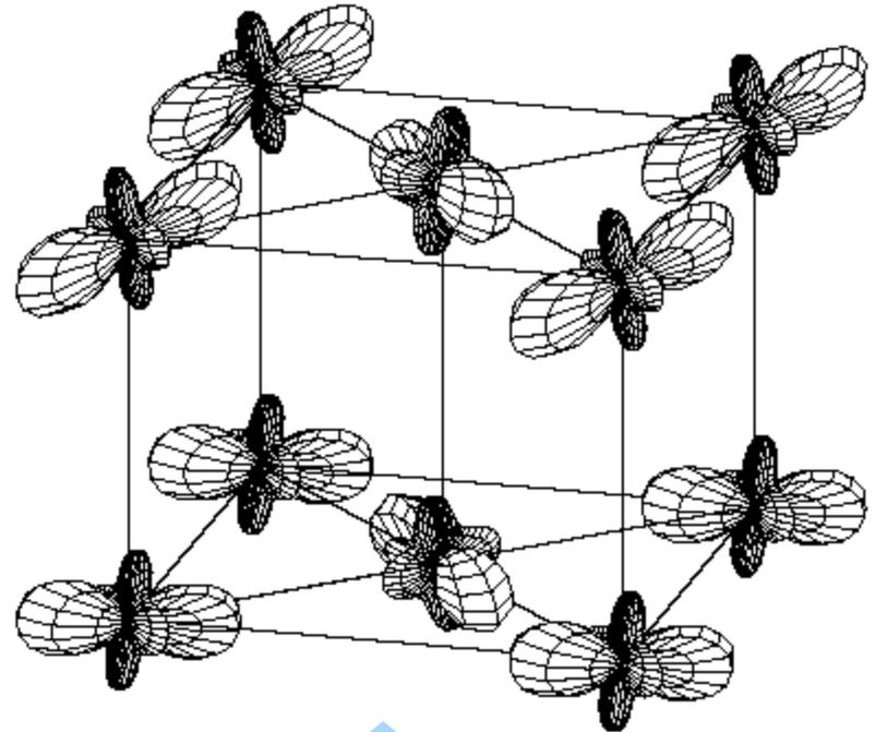
Orbital order for partially filled e<sub>g</sub> shell of Mn<sup>3+</sup> ion in PrMnO<sub>3</sub> in a crystal structure *without* JT-distortion from LDA+U
