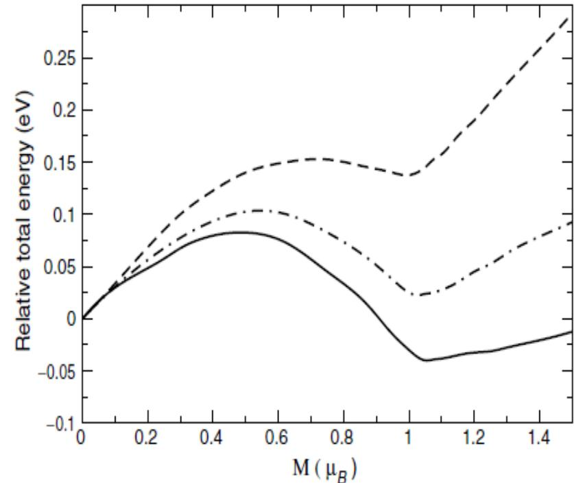
Total energy as a function of the spin moment  $M$ . The solid, dashed, and dash-dotted lines correspond to FeGe, FeSi, and  $\text{FeSi}_{0.58}\text{Ge}_{0.42}$
