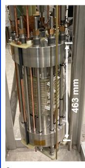
**Figure 1:** Resistive Insulation-Nested Coils (RINC) test magnet containing an inner coil with 12 double-pancake modules and an outer coil with 18 double-pancake modules. The magnet reached 19.2T and studies of quench protection were performed, comprising a demonstration of RINC technology for a 40T all-superconducting magnet.
