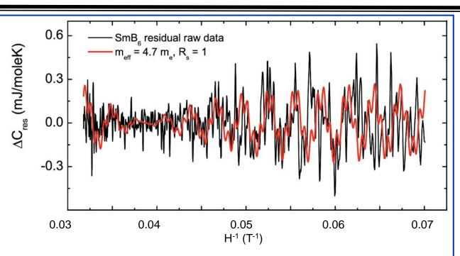
Residual specific heat vs inverse magnetic field (H<sup>-1</sup>) at T=0.58K and  $\Phi$ =45°. The red curve is a comparison of the data to a fit of the L-K model using an effective mass of 4.7 $m_e$  determined from the node in the oscillatory specific heat and the two frequencies of oscillation (341 tesla and 1399 tesla) identified from the Fourier power spectrum at this orientation.
