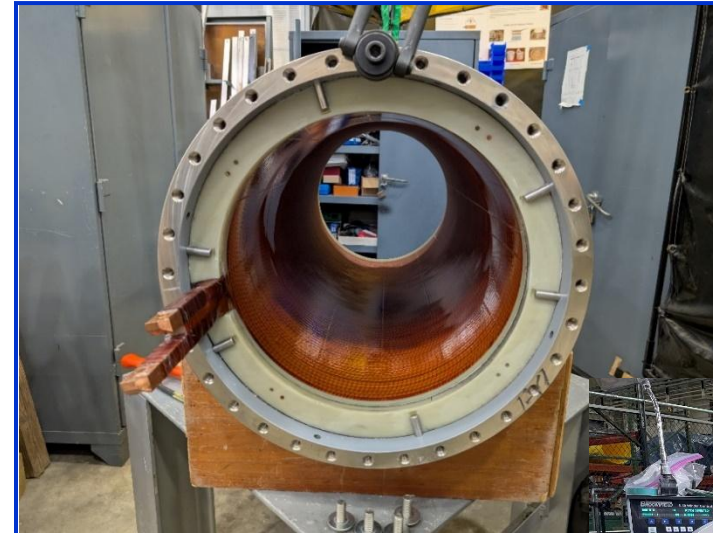
Figure left: View down the bore of coil 7 after epoxy impregnation at FSU. The epoxy impregnation is one of the many detailed procedural steps that includes conductor fabrication, quality control inspections, winding, joint and termination fabrication, outer shell fabrication, epoxy impregnation, Zylon reinforcement application and break out of the coil from the epoxy monolith after impregnation,
