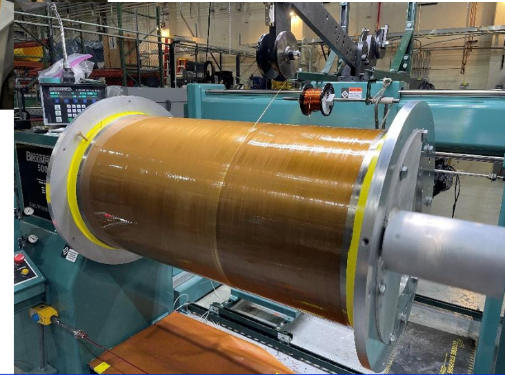
Figure left: View down the bore of coil 7 after epoxy impregnation at FSU. The epoxy impregnation is one of the many detailed procedural steps that includes conductor fabrication, quality control inspections, winding, joint and termination fabrication, outer shell fabrication, epoxy impregnation, Zylon reinforcement application and break out of the coil from the epoxy monolith after impregnation,
