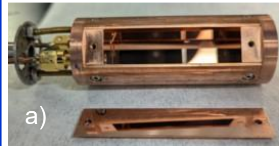
Figure 1(a). A view of the bare Cu cavity with one wall removed. In (b) the cap is lifted showing the internal resonator. The mirror finish is visible in both images.
