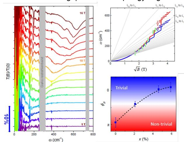
**Fig.1** Dirac mass generation upon finite Fermi level and Cr doping. a, magneto-optical spectrum of undoped  $\text{Cd}_3\text{As}_2$ . b, quantum-to-classical transition at low field. c, Dirac mass acquisition upon Cr doping.
