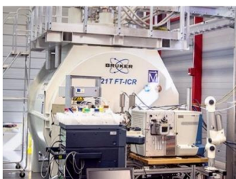
Figure 2.6.1. The MagLab 21T FT-ICR mass spectrometer. Left: previous dual linear ion trap front end. Right: 2024 Eclipse tribrid front end upgrade.
