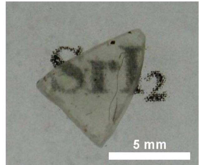
Fig. 5. Translucent ceramic sample of 0.77 mm-thick Eu:SrI<sub>2</sub> backlit.
