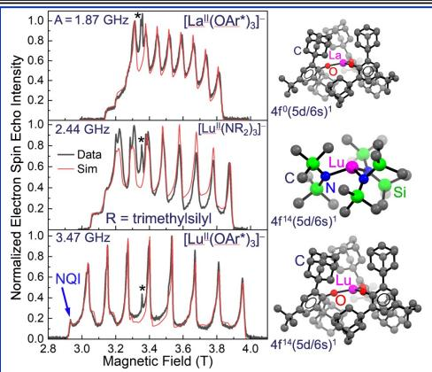
**Figure.** Pulsed electron spin-echo spectra recorded at 94GHz and 5K, for the three compounds shown. The eight (= 2I + 1) lines arise due to the hyperfine interaction (HFI) with the  $I = 7/_2 175$ Lu or 139La nuclear spin; the spacing between peaks is a direct measure of the HFI strength, A, which increases from top to bottom. The asterisk marks an impurity and the "NQI" feature is attributed to a strong nuclear quadrupole interaction.
