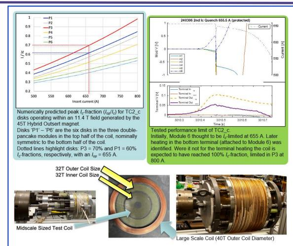
**Facilities and instrumentation used:** ASC/MST Materials Characterization Labs, HTS Winding Shop, DCF 45T Hybrid (outsert) Magnet
