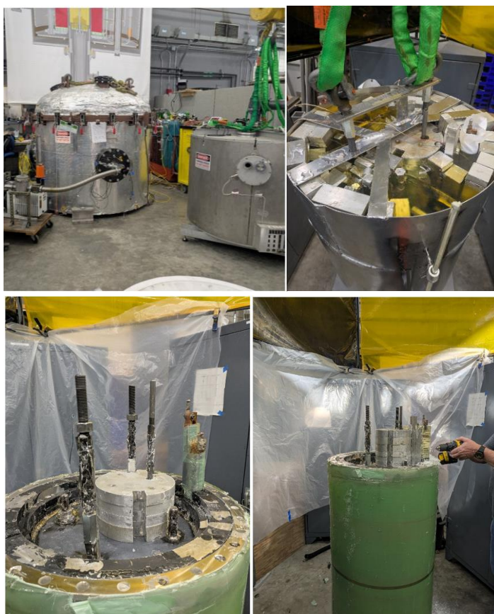
Figure 4.1.14. Coil 7 of the 60T Controlled Waveform (CW) was impregnated in the facility shown on the top left. The top right shows a photo of Coil 7 just after the epoxy curing process. The bottom left and right shown the meticulous “breaking out” of the coil from the surrounding cured epoxy to prepare for final shipment to the MagLab Los Alamos National Laboratory Pulsed Field Facility.
