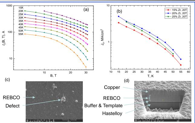
**Figure** (a)  $I_c(B, T)$  for a 4mm wide sample with 20% Zr over 15-55K. (b) Set of critical current density dependencies  $J_c(T)$  for tapes with different Zr doping. (c) SEM top-view image shows a mostly defect-free sample for 20% Zr. (d) SEM view of the conductor cross-section for the sample with 20% Zr.
