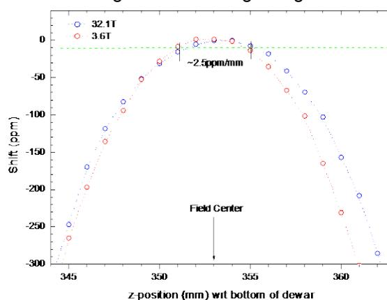
Fig. 1. Field measured with NMR vs. nominal magnetic field. Fig. 2. Homogeneity of the magnetic field near field center.
