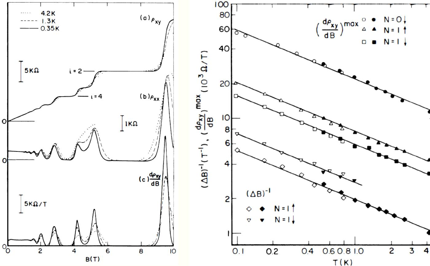
$$\left( \frac{dR_{xy}}{dB} \right)^{\max} \sim T^{-\kappa}, \quad \Delta B \sim T^\kappa, \quad \kappa \approx 0.42 \pm 0.04$$
