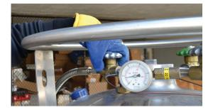
**7** Slowly open the liquid valve, maintaining pressure at about 20 psi — should take 3 to 4 minutes.
