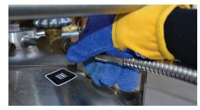
3 Securely attach vent line to vent port on dewar. Open the vent line valve and make sure pressure is below 20 psi.
