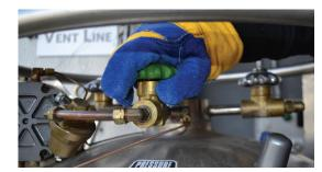
1 Wearing proper PPE, make sure the pressure building valve is closed.
