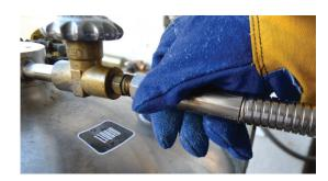
Securely attach the liquid line to the liquid port on the dewar.
