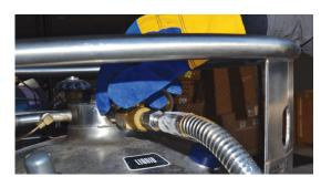
2 Close the liquid valve first, then close the vent valve.
