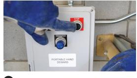
**8** Once filled, press stop button on the portable hand dewar controller.
