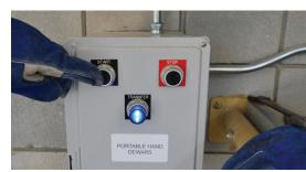
**5** Locate lower controller labeled portable hand dewar. Then press the start button.
