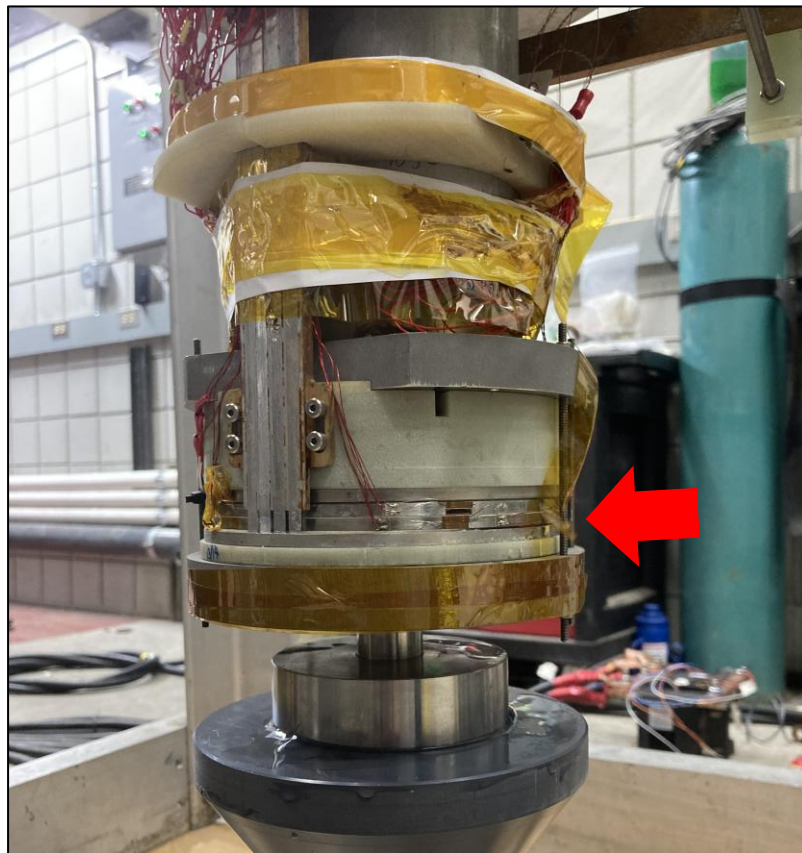
Figure 1 (top): REBCO test coil (red arrow) attached to the load frame that is inserted to test facility at right.
