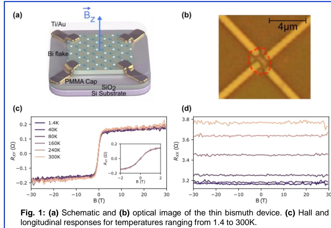
**Fig. 1:** (a) Schematic and (b) optical image of the thin bismuth device. (c) Hall and longitudinal responses for temperatures ranging from 1.4 to 300K.
