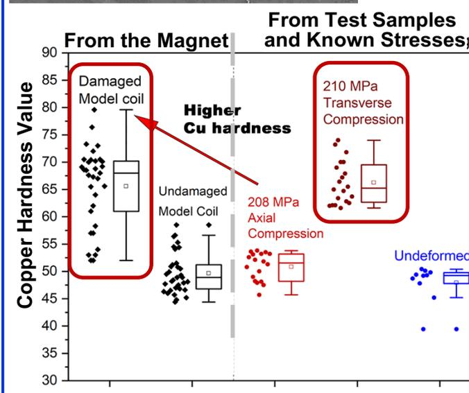
Fig. 2: Comparison of the Cu hardness indicates stresses of over 210 MPa were reached locally in the Nb<sub>3</sub>Sn conductor in the damaged magnet model coil (compare data in two red boxes), resulting in damage to the model coil in the form of Nb<sub>3</sub>Sn filament breakage. A hardness value over 75 in nearby Cu leads to damage in Nb<sub>3</sub>Sn magnets.
