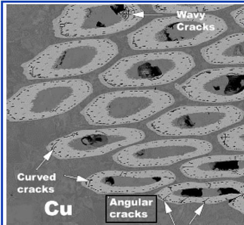
Fig 1: Electron microscope image showing cracks in a conductor that was extracted from a damaged Nb<sub>3</sub>Sn coil that was part of a prototype 11T accelerator dipole magnet built at CERN. The cracks resulted from overstresses experienced during assembly of the model coil.
