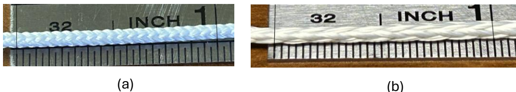
Fig. 4.1.4 (a) 20 PPI coreless braid and (b) 8 PPI coreless braid, both made with 95/5 (95% \text{Al}_2\text{O}_3 , 5% \text{SiO}_2 ) ceramic fibers.
