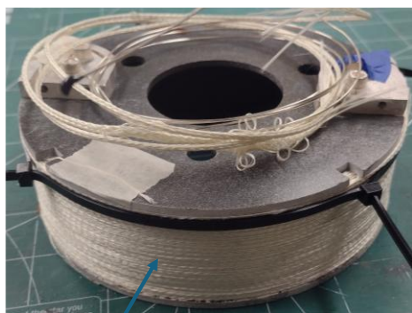
High-strength ceramic fiber reinforced winding pack
