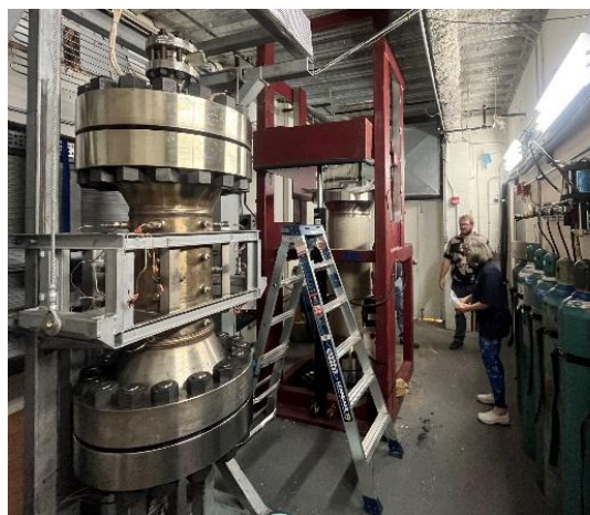
Fig. 4.1.7 ASC's two over-pressure furnaces. The two overpressure heat treatment furnaces for reacting Bi-2212 magnets with the smaller one in the front and the larger one in the rear. A bank of gas bottles that provide the furnaces with a high-pressure gas mix of 98% argon and 2% oxygen can be seen to the right.
