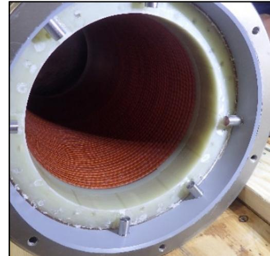
**Right:** View down the 22.5cm diameter bore of the near completed coil, into which the insert coil for the 100T pulsed magnet will fit.
