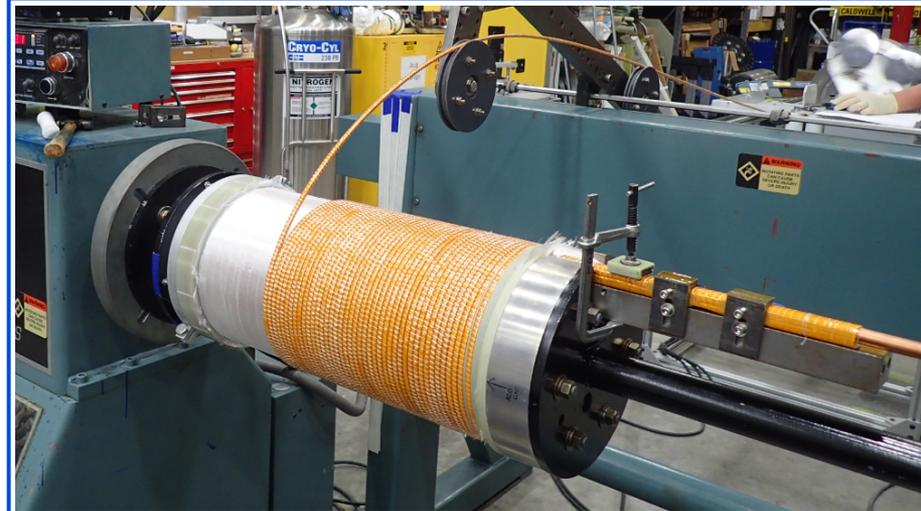
**Above:** Winding of the 65cm long pulsed coil. The leads to and from the coil can be seen extending another 24cm to the right.
