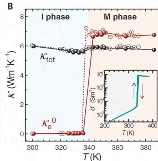
Fig. 1. Thermal conductivity of VO<sub>2</sub> across the metal-insulator transition. (A) False-color scanning
