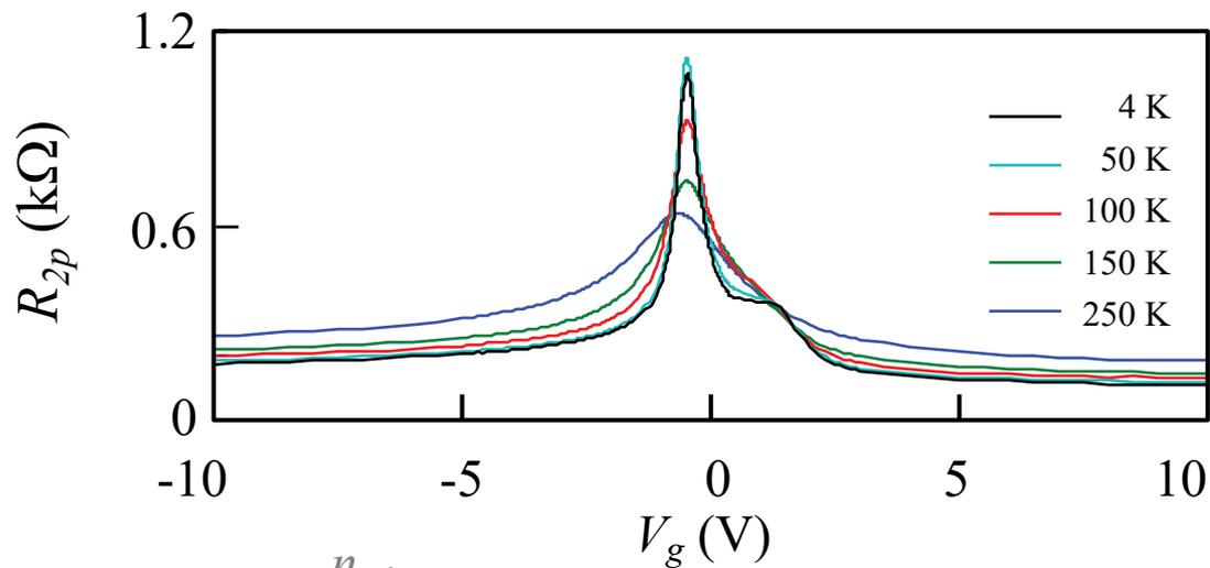
hBN encapsulated single layer graphene
