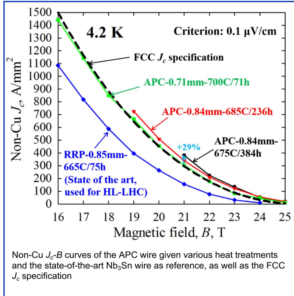
**Facility used:** DC Facility: 31 T resistive magnet (Cell 7).
