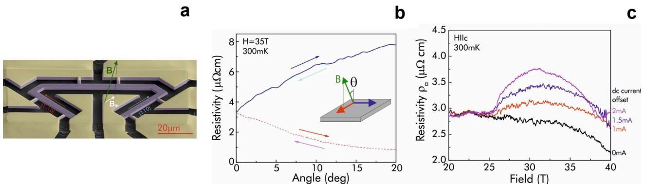
**Fig.1** a) Electron beam micrograph of a CeRhIn<sub>5</sub> microstructure. Current is injected through the bottom contacts and passes the entire U-shaped structure with all three bars in series. b) Angle dependence of the in-plane resistivity at 35T. c) Non-linear conductivity in the high field state.
