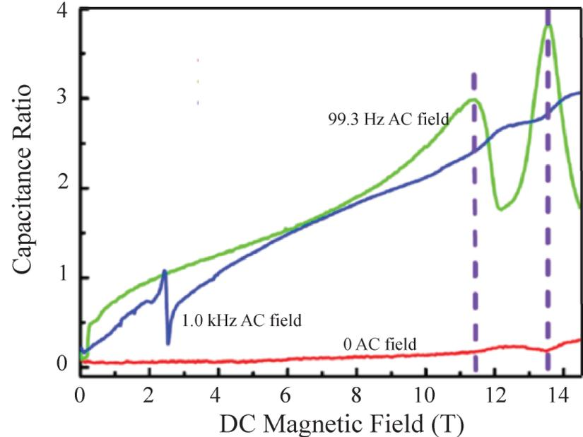
Magnetic field induced changes in the dielectric constant of Br-doped DTN at very low temperatures as a function of applied DC magnetic field at 20 mK [3]. Three changes are observed; (i) a sharp dispersive response at the low critical field ( $B \sim 2.2T$ ), (ii) a peak at the upper critical field ( $B \sim 11.4T$ ), and (iii) a peak at  $B \sim 13.6 T$ , corresponding to the onset of a Mott insulator state.
