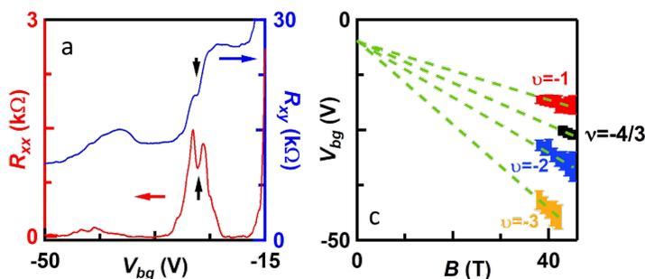
**Fig. 1.** Fractional QH states. Right panel: (a).  $R_{xx}$  (left axis) and  $R_{xy}$  (right axis) of a Hall bar devices  $V_{bg}$  at  $B=45 \text{ T}$ . The fraction QH state manifests as a small plateau in  $R_{xy}$  and an accompanying dip in  $R_{xx}$ , as indicated by the black arrows. Left panels: a constructed Landau fan diagram showing the movement of QH plateaus with magnetic field.
