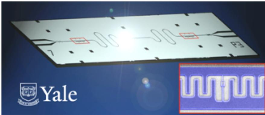
Lithographically produced integrated circuit with semiconductors replaced by superconductors.
