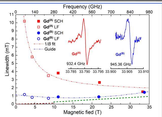
**Figure.** High field EPR linewidth variation with field/frequency, measured in the SCH and a lower-field (LF) spectrometer, for two Gd<sup>III</sup> spin-labels on large biomolecules (Gd<sup>(A)</sup> = Gd[DTPA], Gd<sup>(B)</sup> = Gd[sTPATCN]-SL, see citation). Dashed lines at bottom represent the respective spectrometer resolutions. Representative ultra-high-resolution EPR spectra are shown in the inset.
