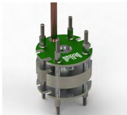
Figure 1: Assembled Open-Source PCB LGR from stackable PCBs.
