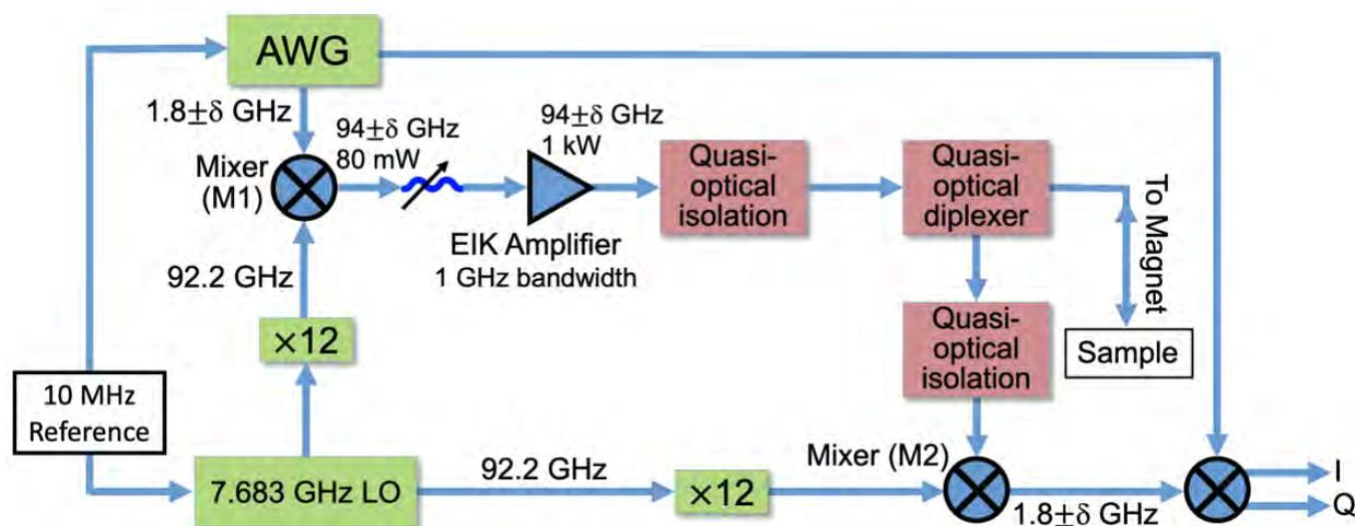
**Figure 1.** A schematic of the AWG implementation in the W-band HiPER spectrometer.
