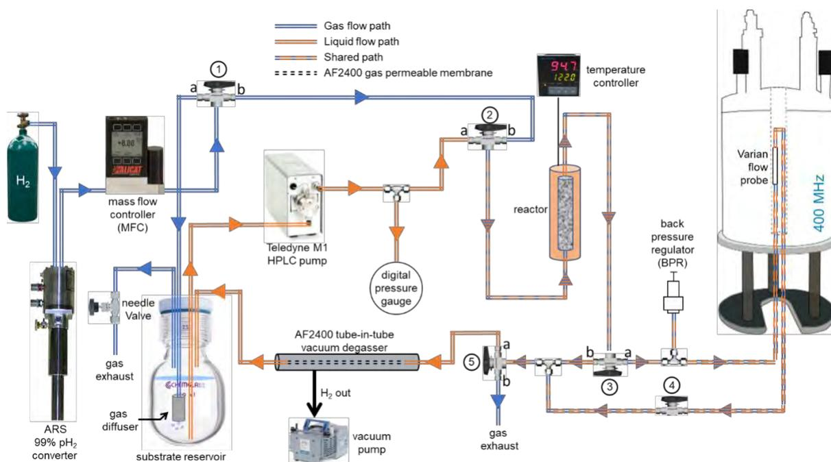
Closed loop continuous flow parahydrogen reactor system. Blue, orange, and alternating double lines represent the flow path of gas, liquid, or both. The grey double dashed line represents the AF-2400 gas permeable membrane in the tube-in-tube vacuum degasser. Arrows indicate the flow direction.
