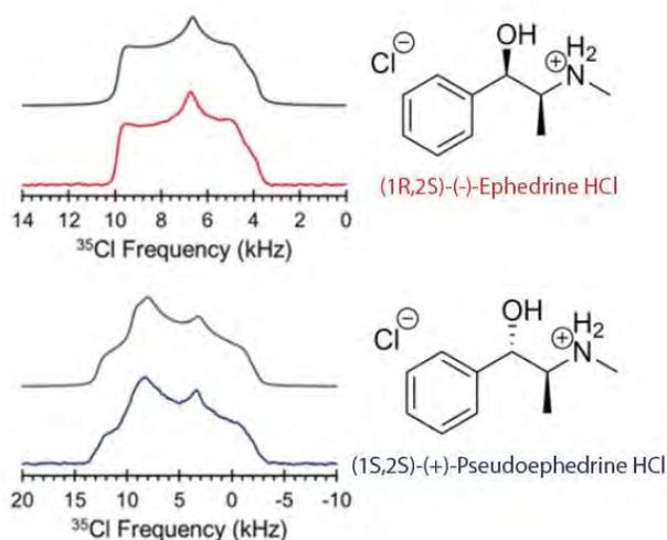
**Figure 1.** Experimental (bottom) and simulated (top) static <sup>35</sup>Cl SSNMR spectra of ephedrine and pseudoephedrine acquired at 21.1 T.
