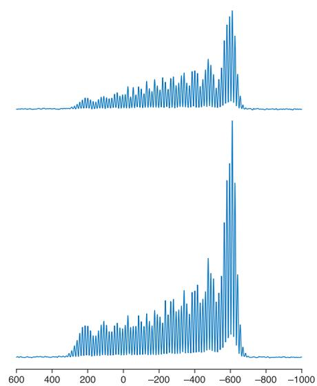
**Figure 1:** Experimental <sup>195</sup>Pt spectra of Pt(NH<sub>3</sub>)<sub>4</sub>Cl<sub>2</sub>·H<sub>2</sub>O acquired using WCPMG (top) and BRAIN-CP (bottom) at a spinning speed of  $\nu_{\text{rot}} = 15$  kHz. Both spectra consist of 256 transients and are acquired at one transmitter offset.
