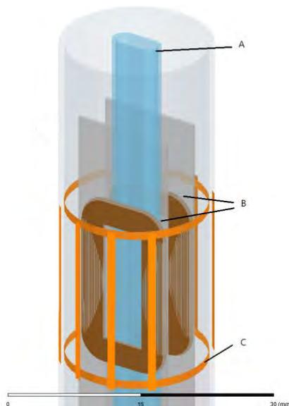
Figure 1: the schematic of the shaped sample tube (A), inner <sup>13</sup>C coils (B) and outer double tuned <sup>1</sup>H/<sup>2</sup>H coil (C)
