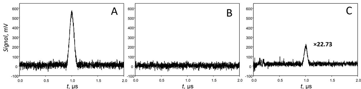
**Figure 1.** A. Single shot 2-pulse spin echo (1  $\mu\text{s}$  delay) measured from 1 mM BDPA in polystyrene (100  $\mu\text{m}$  thick film) using a PBG with  $Q_L=1,538$ . While no echo was observed after the single shot when using  $\text{TE}_{012}$ -type cavity ( $Q_L=1,241$ ) by loading the powdered polymer into i.d.=0.7 mm (B), the signal appeared after 512 averages. All measurements were carried out at room temperature.
