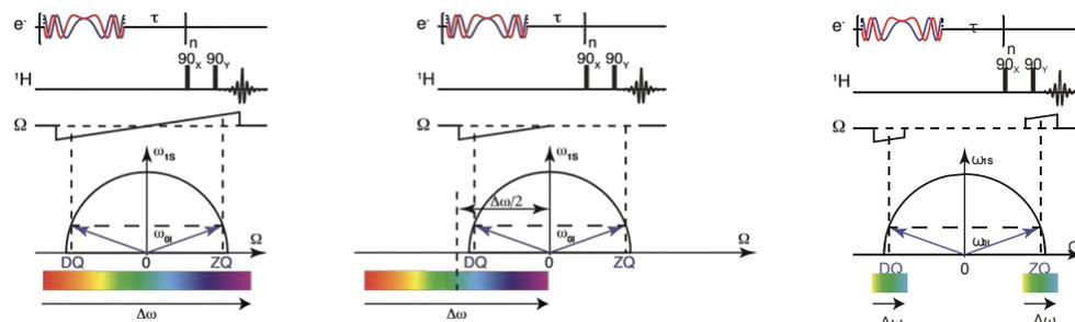
FIG. 1: Schemes of the (a) ISE, (b) SSE and (c) ASE in the rotating frame
