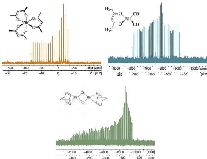
Fig. 1: <sup>1</sup>H-<sup>103</sup>Rh BRAIN-CP/WURST-CPMG spectra acquired at 35.2 T for select Rh-containing compounds.
