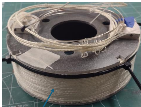
High-strength ceramic fiber reinforced winding pack
