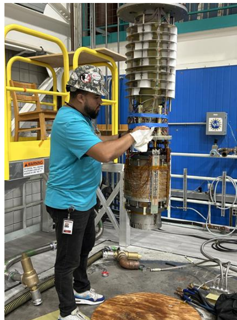
Figure 4.1.19 The LSC1 was being installed for the 2 nd round test.
