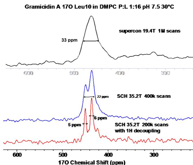
**Fig.1** Comparison of Gramicidin A  $^{17}\text{O}$ Leu10 in DMPC spectra acquired in 19.4T superconducting magnet (black line) and in the 35.2T SCH magnet (blue and red lines). Line narrowing of Leu10 carbonyl oxygen peak reveals the spectra is composed of 2 peaks. Use of weak (30 kHz)  $^1\text{H}$  decoupling reveals line widths ( $\sim 5\text{ppm}$  or  $1\text{kHz}$ ) are dominated by spin-spin relaxation ( $T_2 \sim 360 \mu\text{s}$ ).
