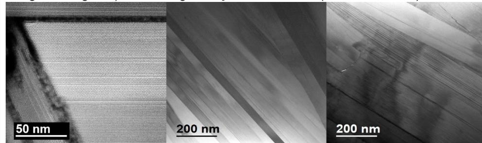
**Figure 2:** Transmission Electron Microscope (TEM) images of the three wires showing grains and grain boundaries. Our results showed that the wire with the lowest  $J_c$  of only 684 A/mm<sup>2</sup> (measured at 4.2K and 15T) had high  $a$ -axis alignment but also had amorphous content at its grain boundaries, which acted as a current transport barrier and thus significantly lowered the  $J_c$  of the wire.
