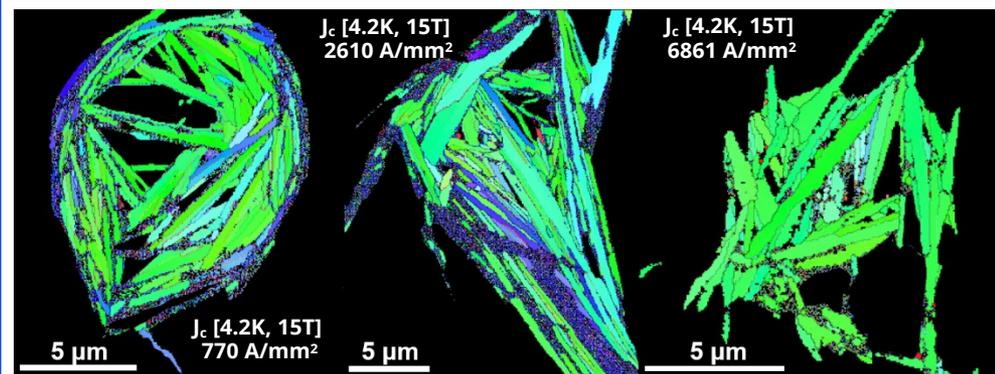
**Figure 1:** Electron micrograph of the cross sections of three Bi-2212 round wires with widely varying critical current densities ( $J_c$ ) showing their  $a$ -axis grain alignments. The wire with the best  $a$ -axis alignment (far right, highest proportion of grains in green) had the highest  $J_c$  of 6861 A/mm<sup>2</sup> (at 4.2K and 15T).
