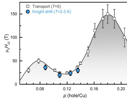
**Fig.1** Saturation field in Knight shift measurements (blue dots, this work) at  $T \sim 2$  K, compared to  $H_{c2}$  values extrapolated to  $T = 0$  from resistivity data [B. Ramshaw *et al.*, Phys. Rev. B 86, 174501 (2012)].
