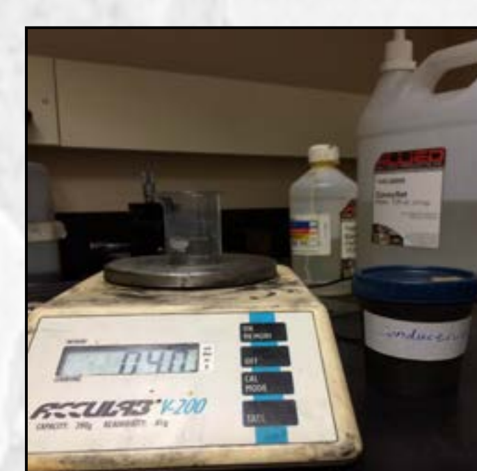
Weighing KonductoMet to make a polymer puck
