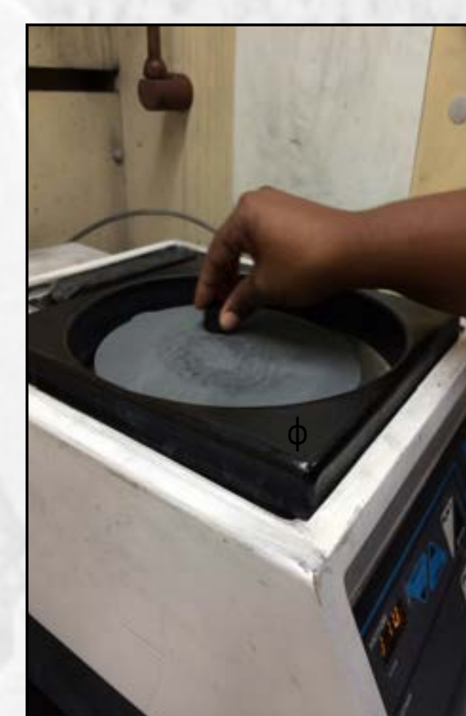
Dry polishing a puck with 400-800 grit silicon carbide paper
