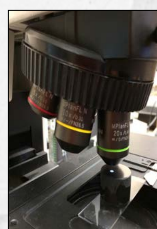
Polished sample ready for image capture and analysis
