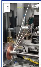
**Fig 1:** Reinforcement is co-wound between each pair of REBCO tapes.
