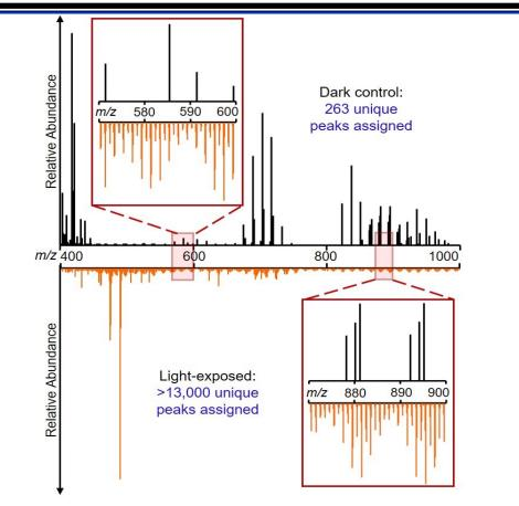
21 T FT-ICR mass spectra of chemicals unique to dark control (black, top) and photoproduced (orange, bottom) for a CVS plastic bag. Thousands of oxygenated compounds were produced by sunlight, compared to only a few hundred that leached in the dark. These results are representative of the trends observed for all plastics tested.
