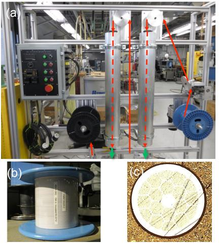
Figure (a) The Bi-2212 insulation system. (b) Insulated conductor on a spool. (c) Cross-section of the 0.8mm diameter Bi-2212 wire featuring a particularly thick layer of insulation.
