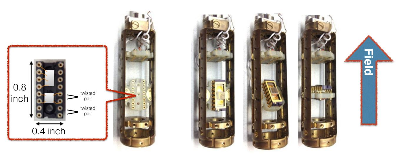
Sample prepared on a standard16 pin dip header can be mounted to a general purpose straight (non-rotating) probe and can be configured to a desired orientation before probe loading, see page 2/2 for proper dip header dimension and shape. Two mini coax cables are also available for the straight probe. For more information including **non-standard sized sample holder** mounting please contact Ju-Hyun Park (jhpark@magnet.fsu.edu)
