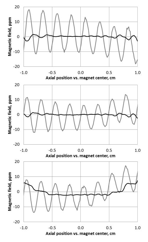
Deviation of field strength along a 1 cm diameter/2.5 mm pitch helical trajectory at 35.2 T, 28.2 T, and 23.5 T (top to bottom): base trajectory (grey) and corrected with combination of passive and active shims (black).
