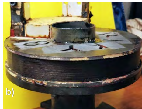
Figure 4.d.9.a, b: Two test coils made with a) aspected conductor made by SMS and b) aspected conductor co-wound with high strengths alloy tape. The high stresses caused the winding pack of coil a) to completely snap at one location.
