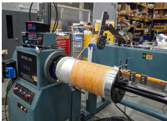
Figure 4.d.16: Winding of Coil #3 of the 100T Outsert.
