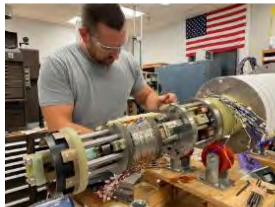
Figure 1. Installing the instrumentation wiring on TC2.
