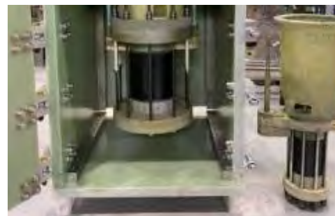
Figure 2. Picture of 85-T magnet mounted in its blast-box. The 65-T workhorse magnet is placed by the side of the box for comparison.
